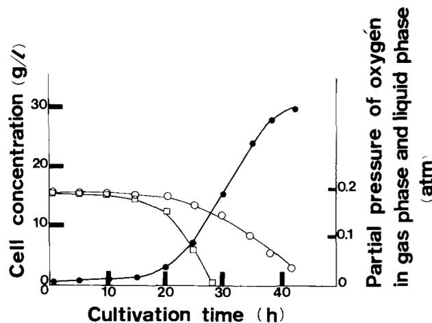
FIG. 1. Autotrophic growth curve of *A. eutrophus* under the gas composition H<sub>2</sub>:O<sub>2</sub>:CO<sub>2</sub>=73.0:10.0:11.0 in recycled gas closed circuit culture system. Symbols: cell concentration (●), partial pressure of oxygen in gas phase (○), and in liquid phase (□).
