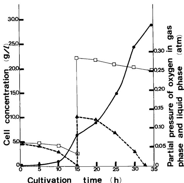
FIG. 5. Effects of gas composition change on microbial growth. Symbols: cell concentration (●), partial pressure of oxygen in gas phase (□), and in liquid phase (▲).
