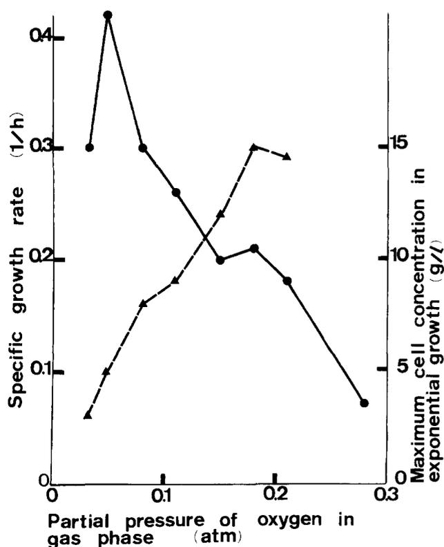
FIG. 3. Effects of partial pressure of oxygen in gas phase on specific growth rate (●) and maximum cell concentration (▲) in exponential growth phase.
