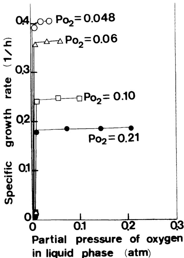
FIG. 4. Effects of partial pressure of oxygen in liquid phase on specific growth rate.
