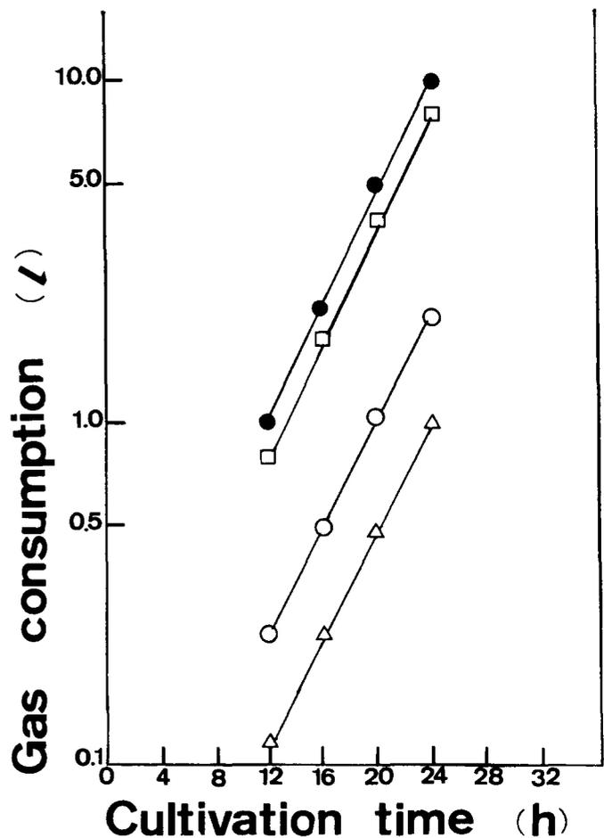
FIG. 2. Linear relationship of gas consumption increase during culture. Symbols: hydrogen (□), oxygen (○), carbon dioxide (△), and gas mixture (●).
