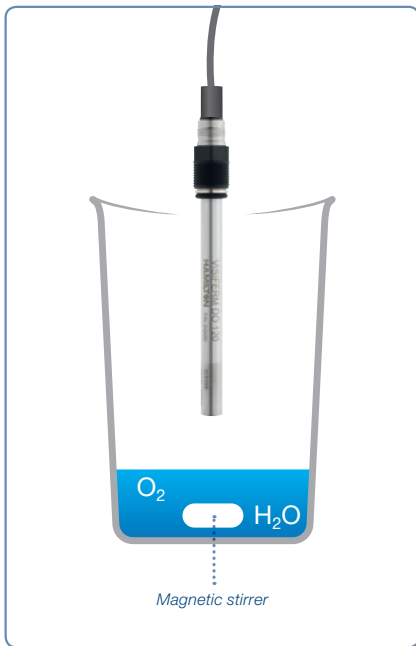
Figure 22: Calibration setup in saturated medium.
